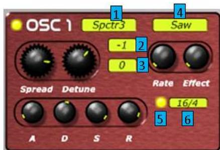
The main feature of the Oscillator section is its unique 14 Oscillator detuning algorithm. Detuning creates many 'copies' of the sound waveform at a slightly different pitch, ending up in a much fuller, fatter sound. It is comparable with a choir in which many voices of different pitches add up to form a 'wall of sound'.
