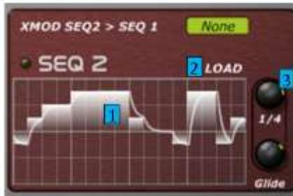
Gemini's sequencers can be programmed simply by clicking on the notes in the sequencer grid [1]. Alternatively preprogrammed waveforms from **ROM** can be loaded [2]. Make sure that the sequencer has been enabled. (Click LED on)
