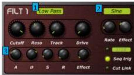
Gemini sports 2 high quality analogue modeled filters. They can be used for each oscillator section separately to create true stereo effects (parallel mode) or they can be used in serial mode.
